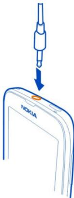
Do not connect products that create an output signal, as this may damage the device. Do not connect any voltage source to the audio connector. If you connect an external
