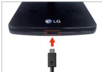
**NOTE** Fully charge the battery before initial use of the phone to maximize the battery's lifetime.
